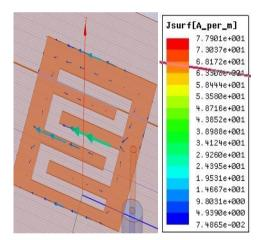
Figure 14: Current distribution at vector\_Jsurf
