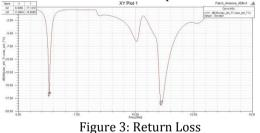
From the figure 3, the return losses of the proposed antenna at 6.3065GHz and 11.0804GHz are -17.1318dB and -18.8089dB.
