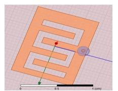
Figure 1: geometry of rectangular probe-fed with folded dipole.
