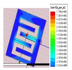
Figure 13: Current distribution at mag\_Jsurf
