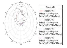
Figure 7:Radiation pattern phi
